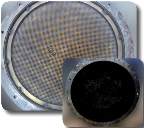
A damaged and a dirty filter.
